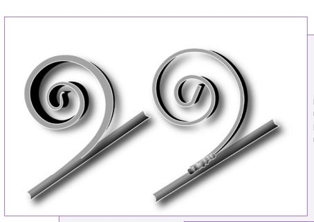
Right, leaf detail fire-welded to a round bar.
