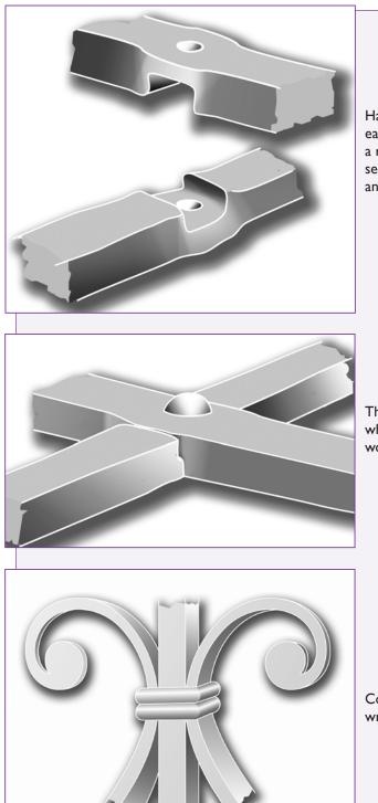
Halving is used where bars are lapped over each other, or where two pieces are joined for a run longer than the stock. These joints can be secured by rivets, which may be countersunk and difficult to see under layers of paint.
