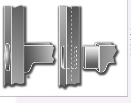
Far left, forged scroll fire-welded to a round bar. Right, cold-bent scroll arc welded to a round bar.
