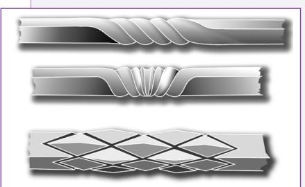
Top, simple cold twist. Middle, progressive reverse twist, made hot.
